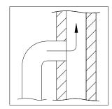
The wood burning stove can be connected to a chimney to which other heat sources are connected.
